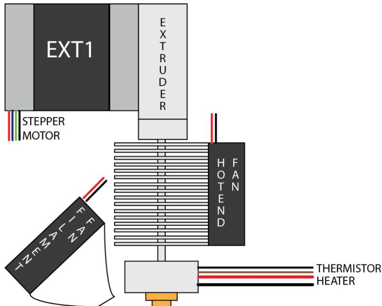
This image shows a normal direct drive extruder/hotend setup. If Bowden is used the setup is almost the same, but there is a tube between the extruder and hotend.
