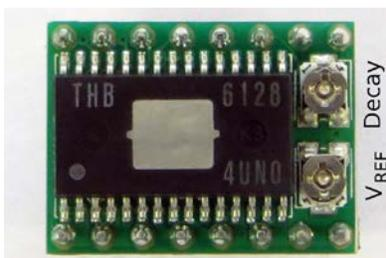
By turning the decay potentiometer, the way of voltage and current decay in the motor coils is changed. A medium setting has been proven to work with many Nema 17 motors."
