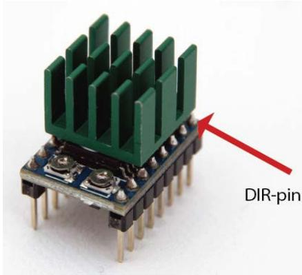
When you orientate the RAPS128 like in the image, the DIR pin is in the upper right corner
