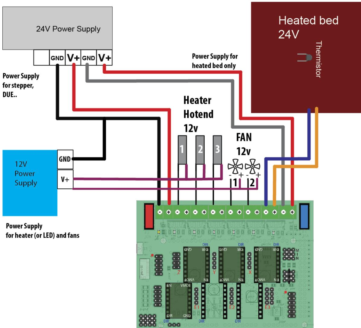
RADDs do switch the negative side. Sample: To turn on Fan 1 RADDs switches the negative fan pin to GND. The positive fan wire is connected to +12V so the fan start.
