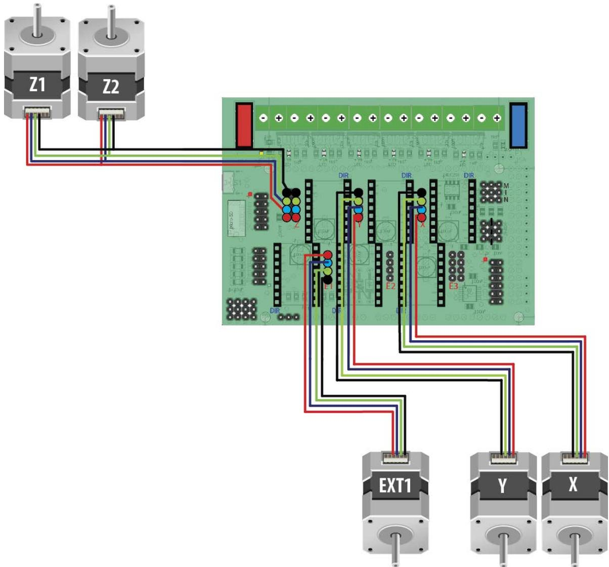
Sample: A setup where you use dual stepper motors for the Z-axis, X and Y-axis + one extruder. This is a normal setup on many printers.
