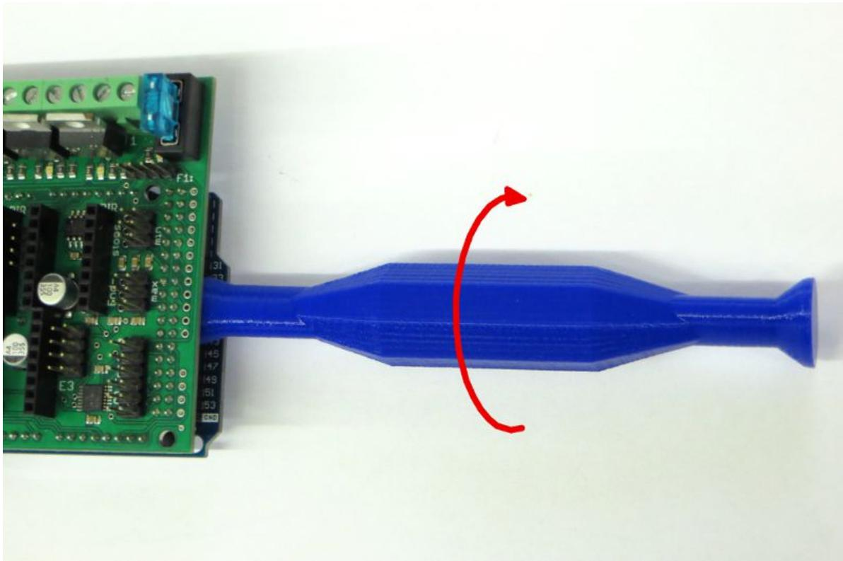
By using this tool, you can remove the RADDs board without making any damages.
