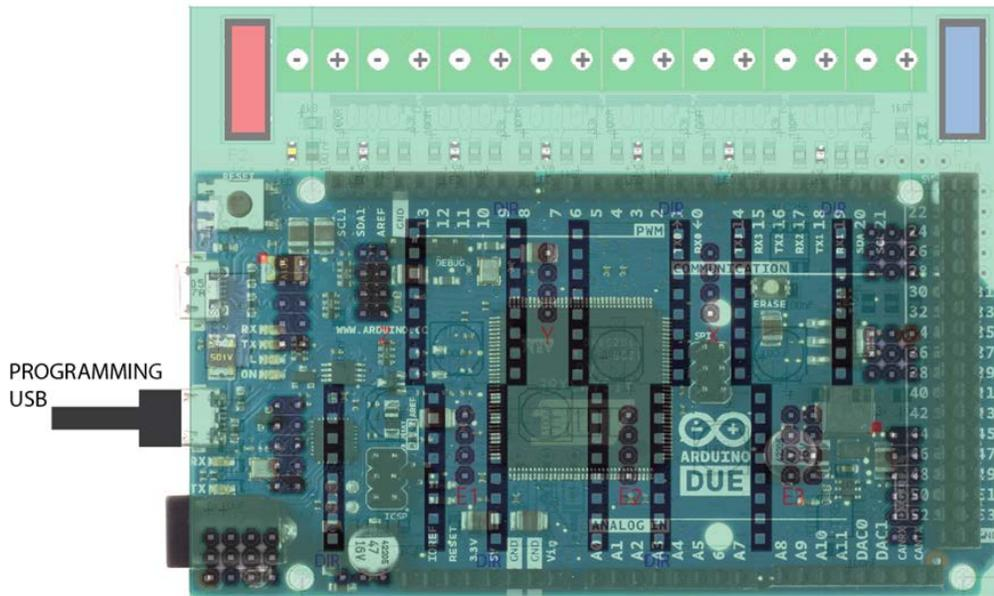
Mount the RADDs board on the top of the Arduino DUE.
