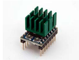
**CAUTION:** Inverted activation signal Enable = HIGH (at Pololu drivers enable = LOW, invert in firmware!)
