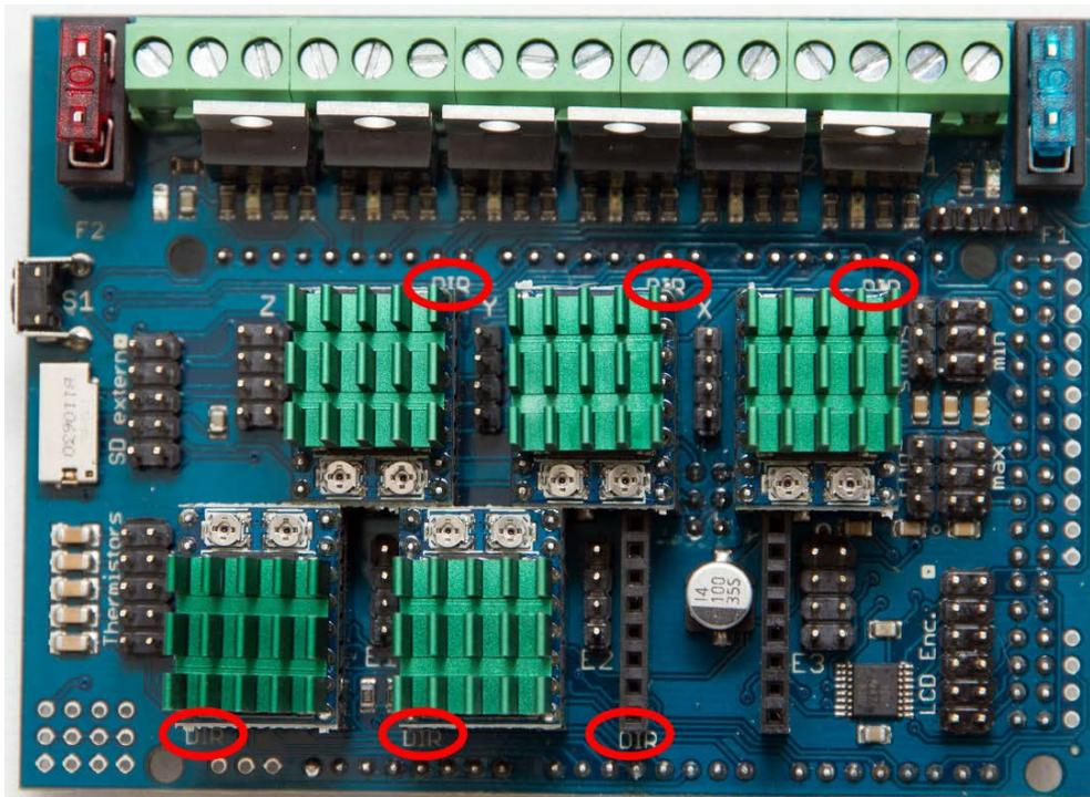
When you insert the stepper drivers, the drivers DIR pin have to point towards the DIR label on the RADDs driver socket.
