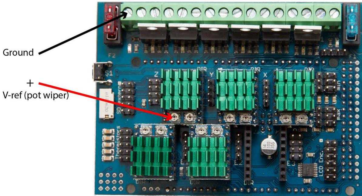
The arrows indicate the measurement points for the reference voltage. Use a voltmeter and measure the voltage between the ground terminal and the pot wiper on the driver's v-ref potentiometer.
