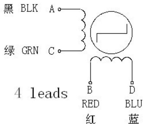
Wiring diagram for Wantai 42BYGHW609 stepper motor (from [www.wantamotor.com](http://www.wantamotor.com)).
