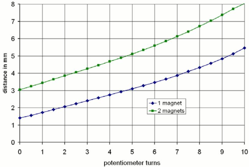
The spindle potentiometer has 10 turns and 10 kOhms. One turn corresponds to 1 kOhm. The potentiometer on the circuit board has 5 kOhm and a corresponding adjustment from 1.4 to 3.1 mm (one neodymium magnet N45 with D = 4 and H = 1).
