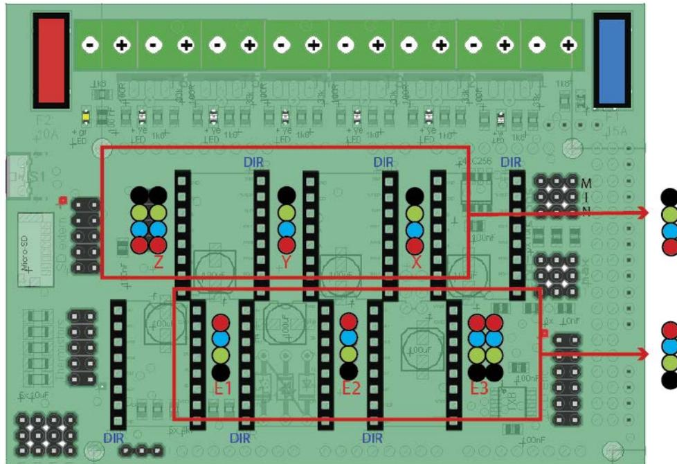
The Z and E3 axis comes with dual motor pin connections so you can connect an additional stepper easily on these axis..
